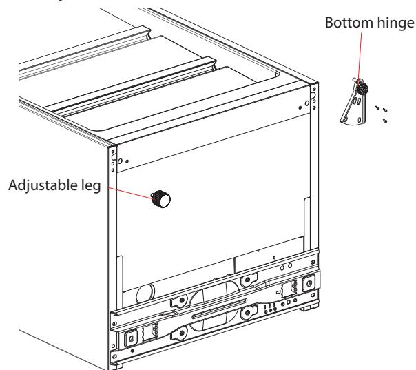
6. Install the lower hinge on the left side of the freezer and the adjustable leg on the right.
