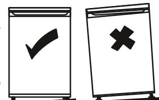
**Note:** Ask a second person to tilt the freezer backwards to ease the setting of the foot. Perform this operation before placing the food in the freezer.
