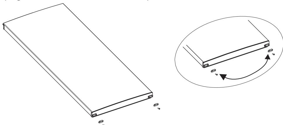
5. Remove the lower hinge and an adjustable foot.
