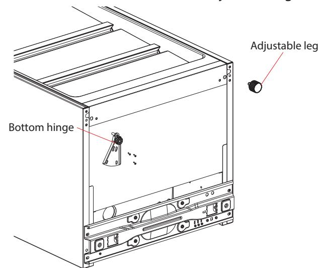
7. Install the door on the lower hinge and check that the seal is sealing properly and that the door position is correct. Install the left upper hinge and attach the cover to the hinge (supplied as an accessory). Finally, attach the cover to the holes for the right upper hinge.
